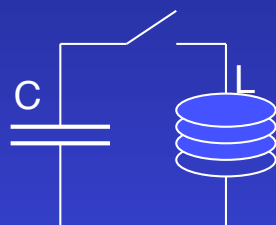
Pulsed magnetic fields are generated by LC circuit
